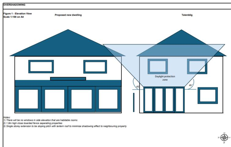
**Fig. 3 - DRAWINGS SUBMITTED WITH P/24/541/OUT SHOWING DAYLIGHT PROTECTION ZONE**
